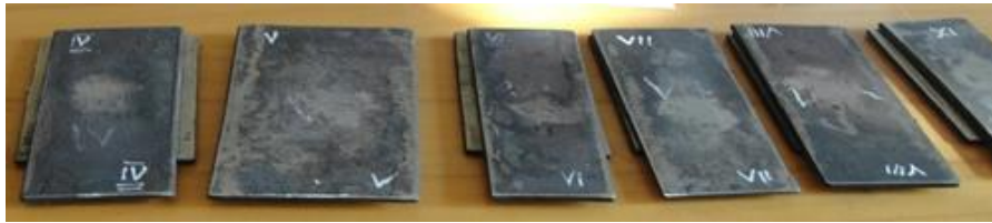
Fig. 4. Explosive-welded steel plates of different hardness
